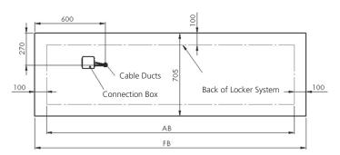
Baseplate with connection box\* for electricity and internet for use of between 11 to 20 cabinet modules.
